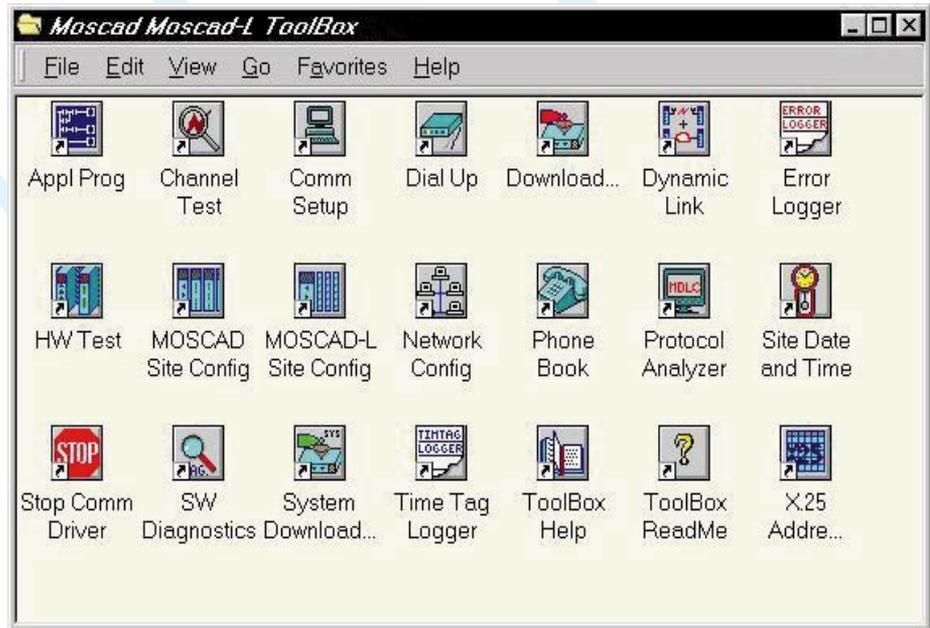
ToolBox programs run on a PC Pentium platform using Windows 95™ or Windows NT™ operating system. The user may connect his PC to any site in the network in order to remotely set up, diagnose or reprogram any of the system's MOSCAD or MOSCAD-L RTUs.
