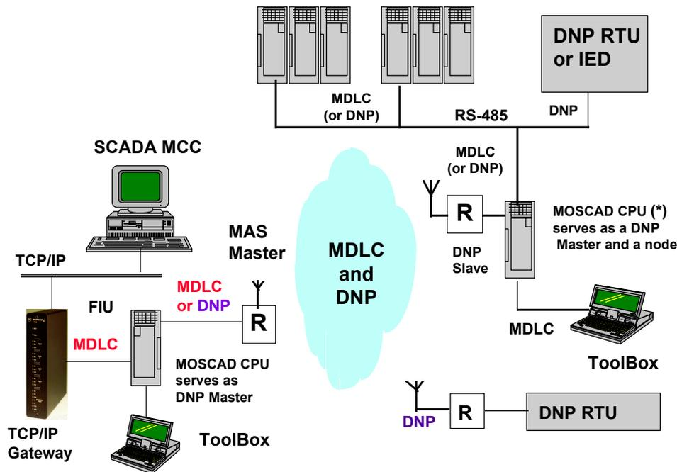
Figure 2. DNP capable RTUs in MOSCAD Environment
