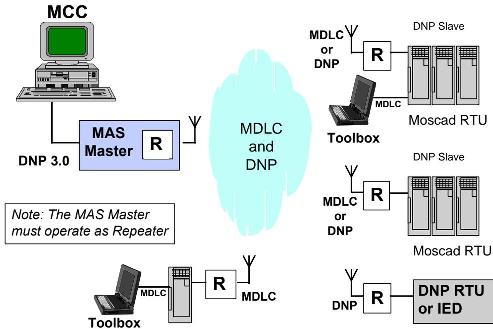
Figure 1. Implementation of the DNP-3.0 concept using MAS radios.
