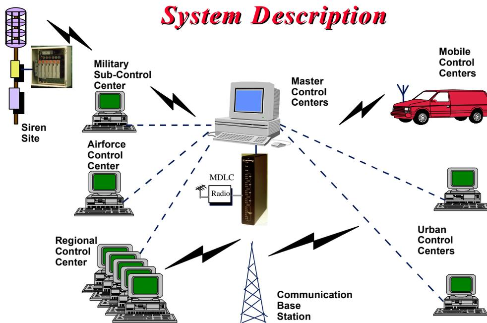
Figure 1. Siren System Diagram
