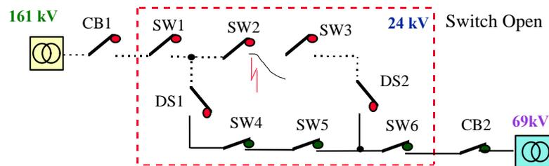
Figure 3 d. Fault Isolation Process
