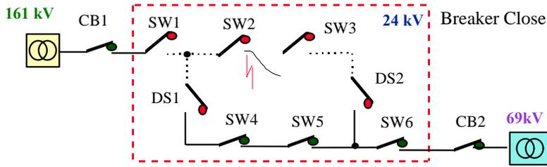
Some 30 seconds after the last attempt (programmable interval), the CB “re-closes” again. Since the other switches, SW1-SW3, remain open, the CB may “re-close” and allow renewed supply of power to customers.
