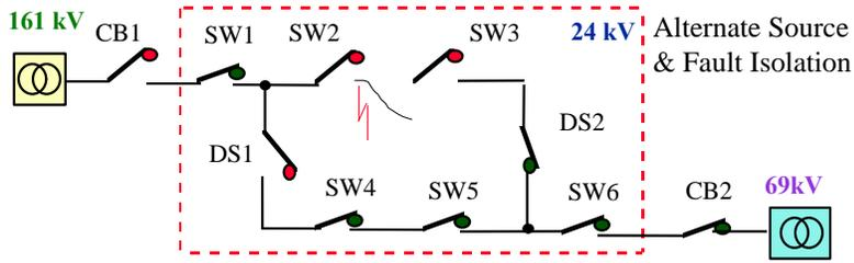
Following closing the DS2 switch all customers (except those connected SW2 - SW3 section) will receive power. The DS2 reconnection (performed by the operator) may take few minutes.
