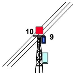
The RTU is powered from a 110V transformer (item 9). The same AC input also serves for fault detection purposes.
