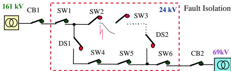
The RTU controlling SW2 now “understands” that the fault is located close by, thus it will immediately re-open the switch. The switch remains open, ensuring that the fault is isolated.
