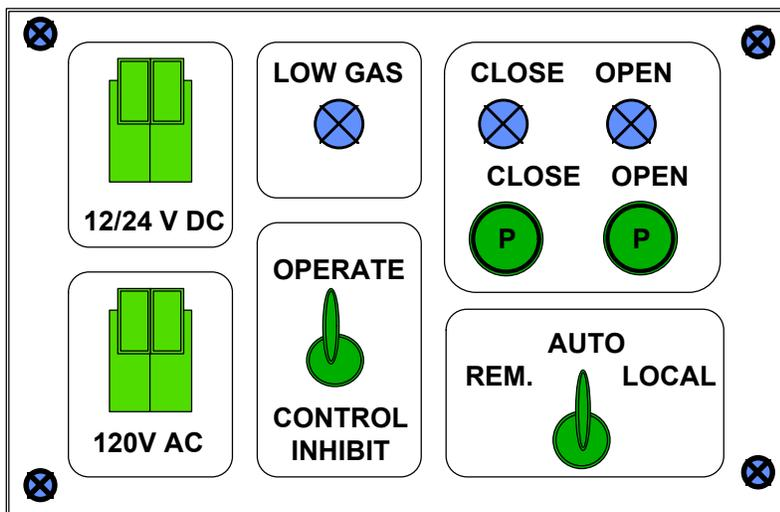
The RTU control panel serves for human interface. Operation of the lamps, are subject to opening of the RTU door.
