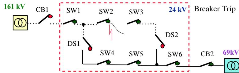
Figure 3 c. Power fail to the whole network
