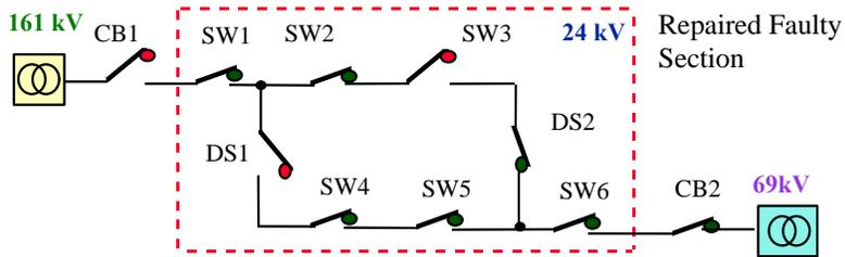
After completion of the repair (which might take a day or even longer), power is restored to all customers. The grid may remain in its new configuration, or be restored to the original one.
