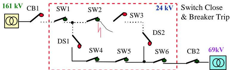
Some 90 seconds after opening of SW2, its RTU will “re-close” the switch. Since the fault is between SW2 and SW3, this attempt results in tripping of CB1 at the substation.
