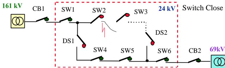
Some 60 seconds after the opening of SW1, its RTU will “re-close” the switch. Since switch SW 2 is open, and the fault between SW2 and SW3 is isolated, the power is restored.
