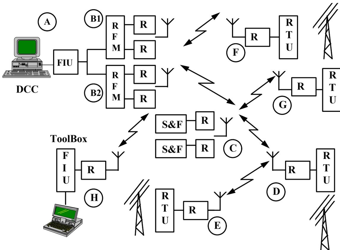
Figure 2. IEC System concept for a single region
