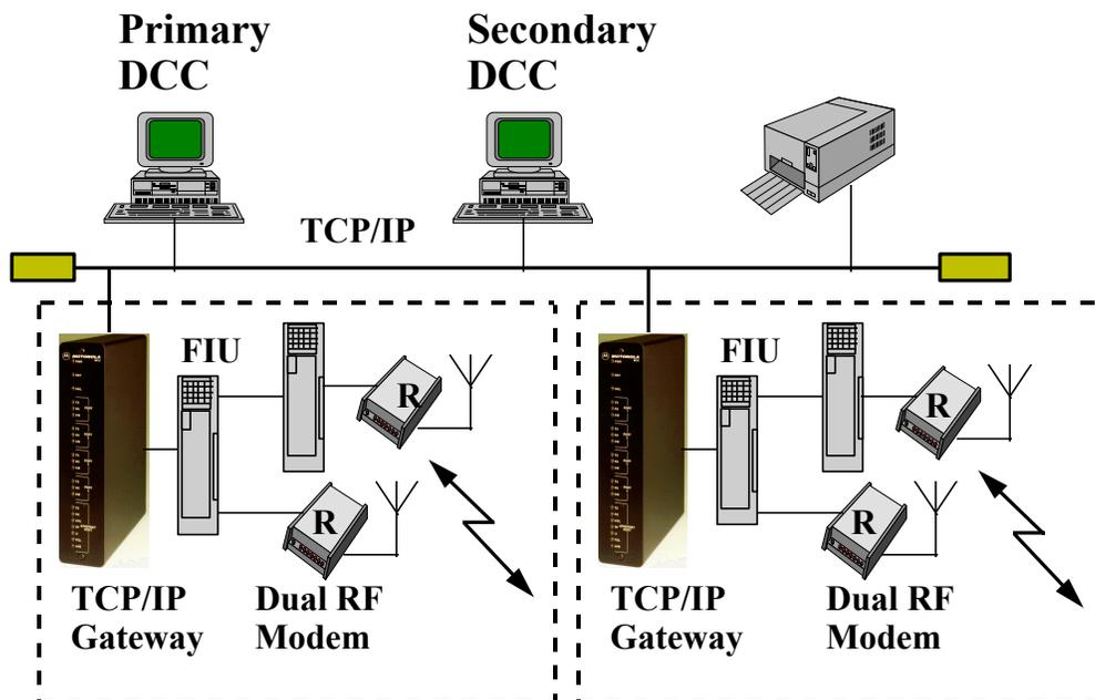
Figure 5. Full Redundant DCC Interface
