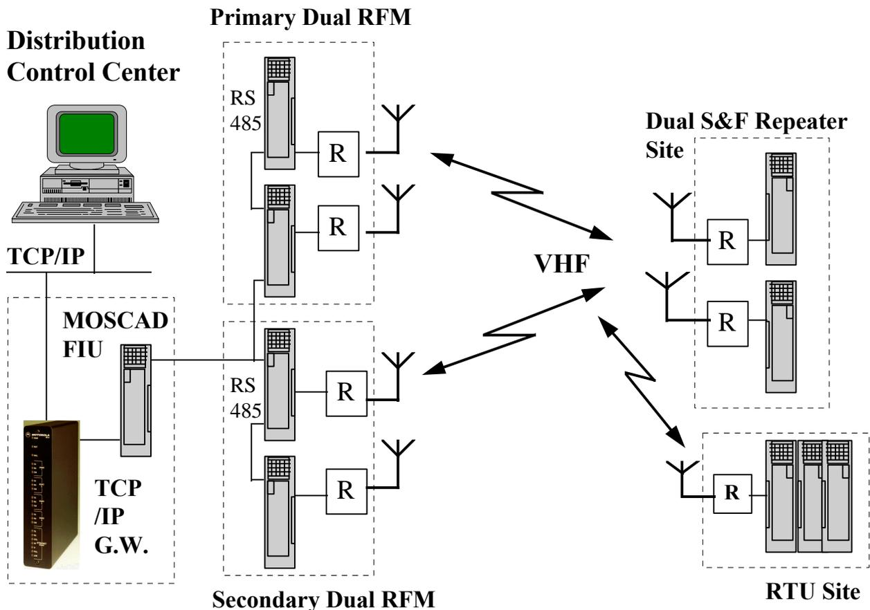
Figure 1. Illustration of Communication Links
