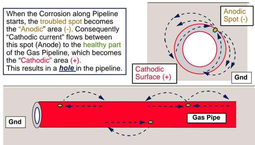
Figure 1. Destructive Corrosion Current
