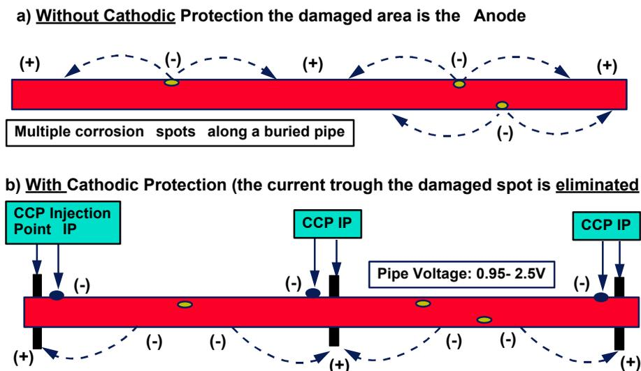
Figure 3. Implementation of Cathodic protection
