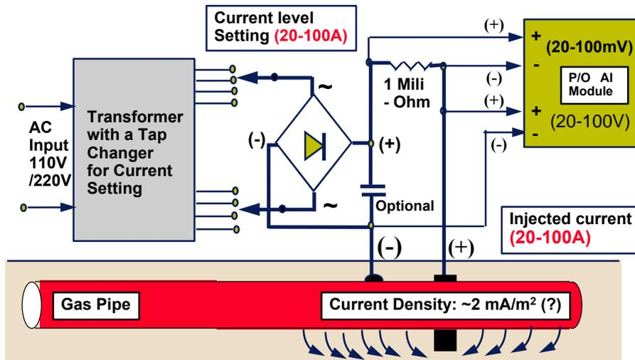
Figure 4. Cathodic Protection system
