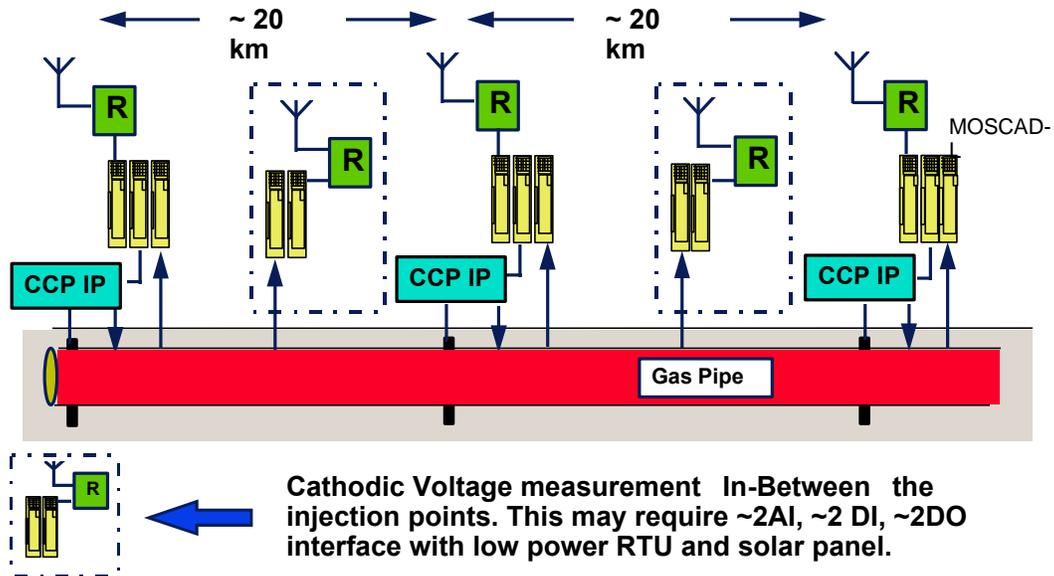
Figure 6. Enhanced measurement along the pipeline
