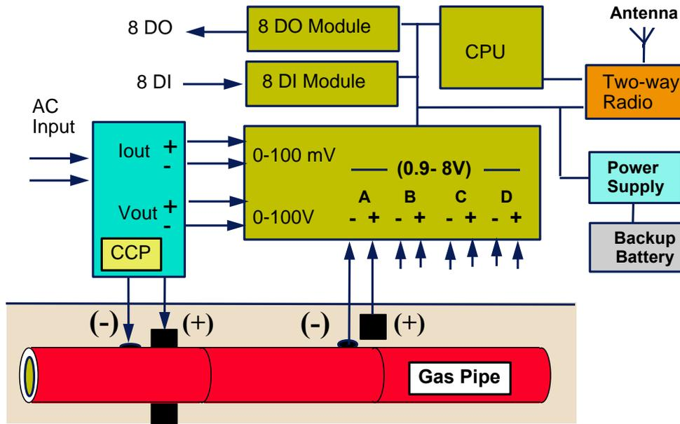
Figure 5. RTU Connection for CCP Monitoring
