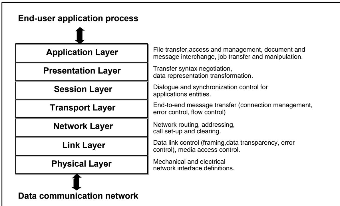
Figure 1. OSI/ISO protocol structure
