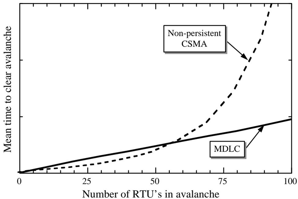
Figure 5. MDLC vs. non-persistent CSMA
