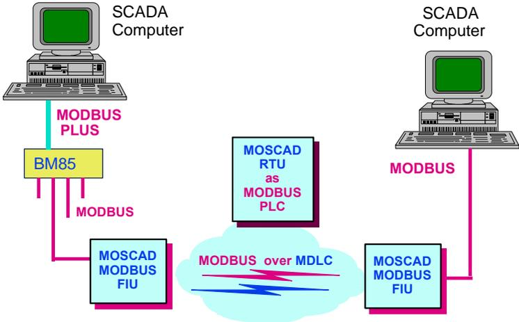
Figure 6. MODBUS type Interface to a Wireless System
