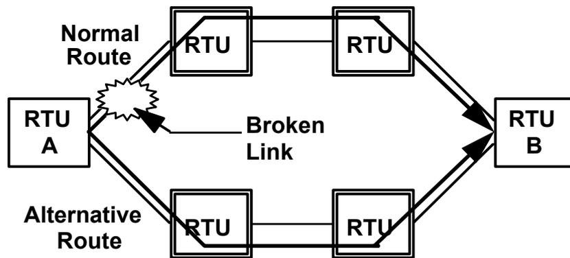
Figure 2. Communication path restructure
