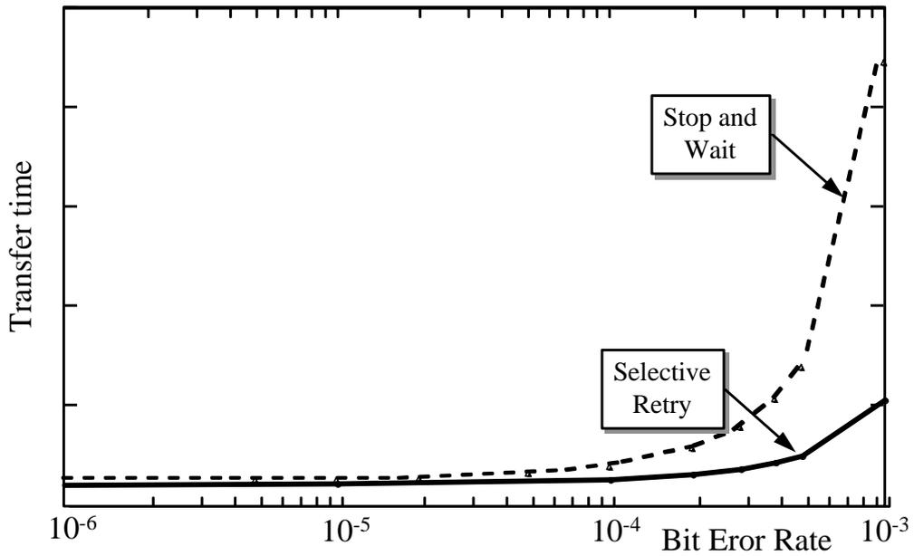
Figure 3. Selective re-transmissions versus stop-and-wait.
