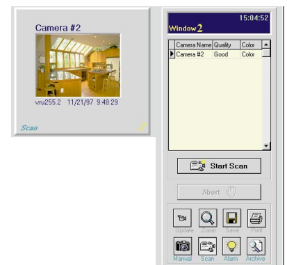
Figure 9. Control Panel for Scan Mode
