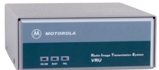
Figure 2. VRU in Desktop Enclosure
