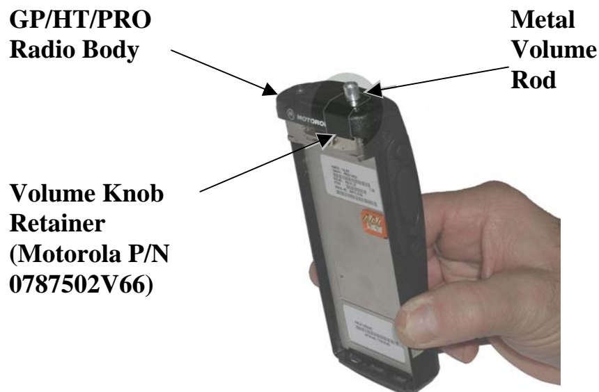
Figure 11-23 Attach Retainer to Radio
