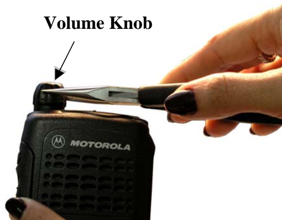
Figure 11-21 Removing the Volume Knob
